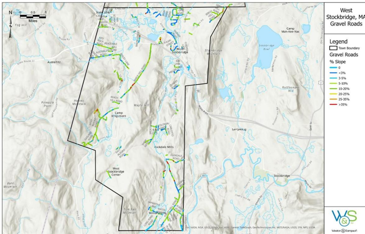
Figure 2. Slope of Gravel Roads in West Stockbridge
